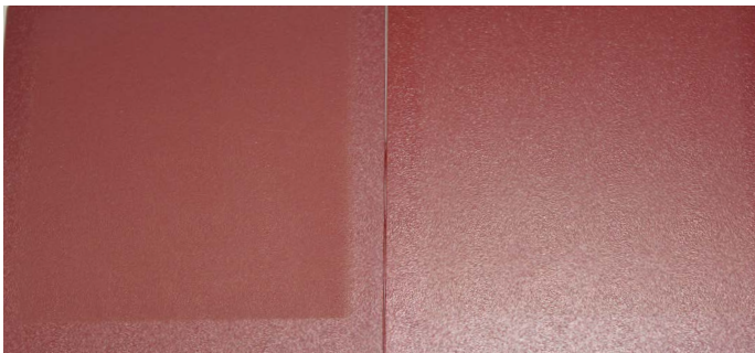
Gloss retention - Accelerated weathering QUVB 600h - Alesta® AP left/ Alesta® SD right
