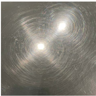
Sensitive dark, glossy finish 80GU after Martindale test
