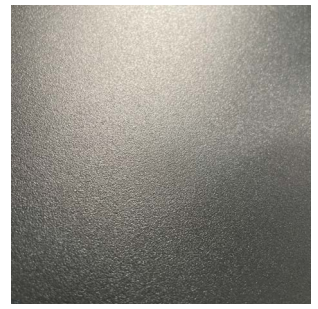
Alesta® SD Fine textured finish 5GU after Martindale test
